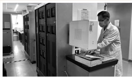
In the Diagnostic Bacteriology Laboratory, MLT Yap Hock Guan loads a random-access automated PCR test for SARS-CoV-2 into a machine that is also used for Methicillin-resistant *Staphylococcus aureus* and carbapenemase-producing *Enterobacterales* screening.
