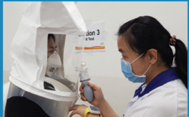
Ensuring a proper fit between the mask and face with the use of a bitter solution – if the user does not detect the taste of the solution, the fit is acceptable.
